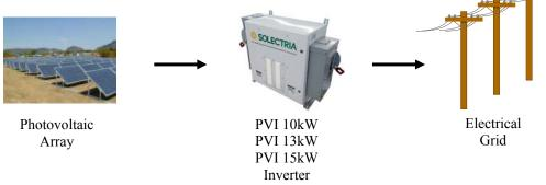
Fig. 1 Grid tied inverter application
