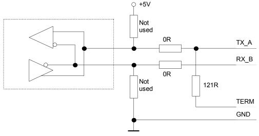
Representative RS485 schematic, inside the inverter
