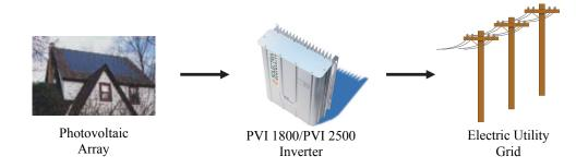
Fig. 1 Grid tied inverter application
