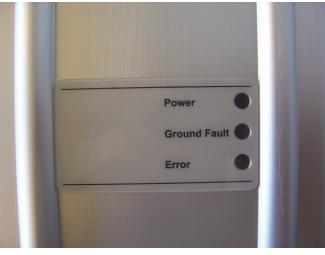
Fig. 8: Power, Ground Fault and Error Indicator
