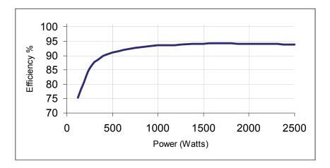
Fig. 13b PVI 2500 efficiency plot
