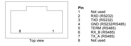
Hint! Both RJ45 connectors have the same pin-out. Use RJ45 crimping tool such as AMP/Tyco Electronics P/N 2-231652-0 Other versions of RJ45 crimping tools are also available at stores such as Radio Shack.
