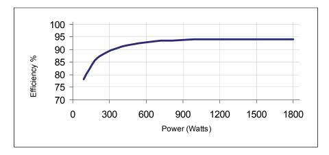
Fig. 13a PVI 1800 efficiency plot
