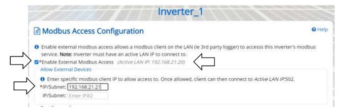
Figure 3-28 Enabling external Modbus access, Port Forwarding
