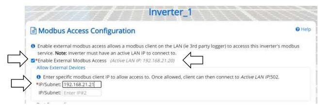
Figure 3-29 Enabling external Modbus access, static routing
